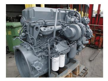
When Requested these running engines bottom ends are gone through and New Connecting Rod Bearings, Main Bearings, Thrust Washer, Front & Rear main seals, Oil Pan Gasket & Filters are replaced with New. The Engines are then cleaned and painted and then run Tested again.
